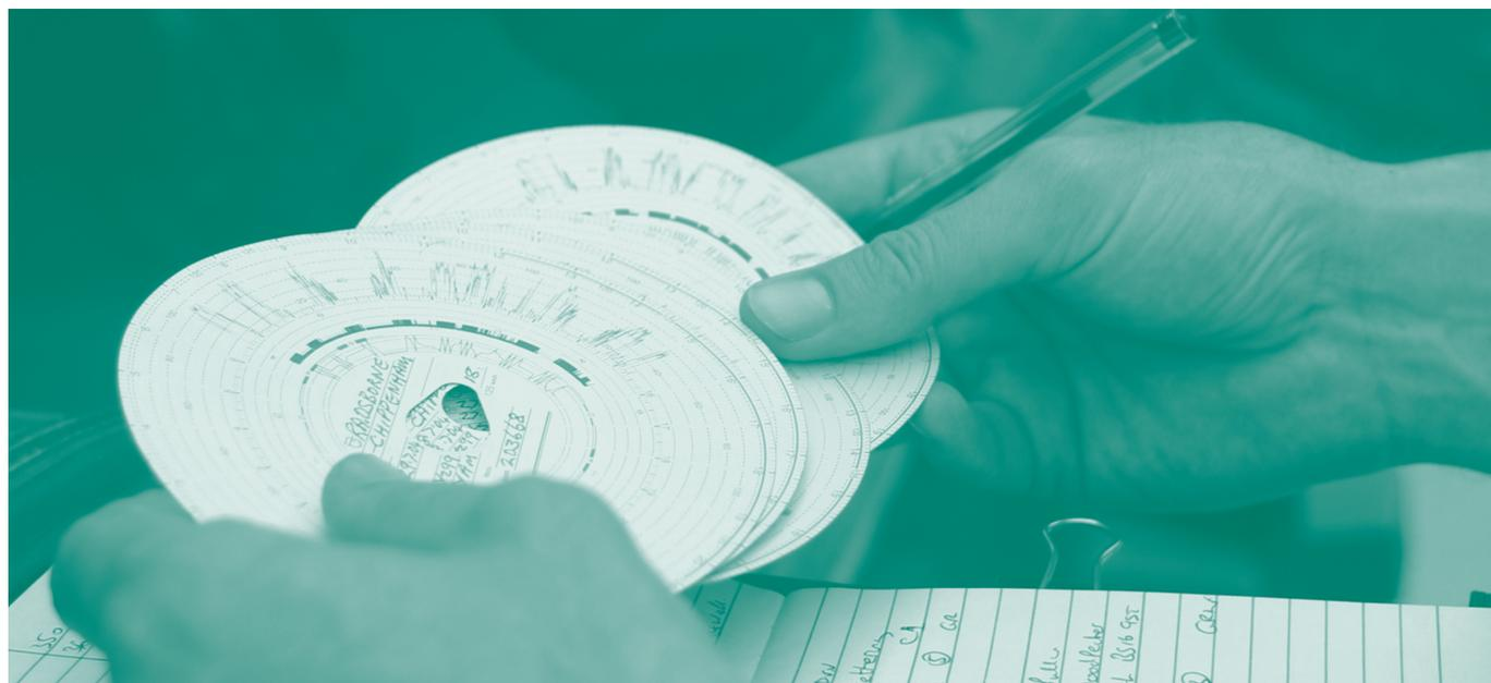
An approved tachograph is the required instrument by which the activities of drivers subject to the EU or AETR drivers' hours rules, and the vehicle's speed, distance and time are recorded. There are two main types of tachograph – analogue and digital. The only exception is when driving a vehicle engaged in the collecting of sea coal. In this one case you are subject to the EU rules on drivers' hours but do not need a tachograph.
