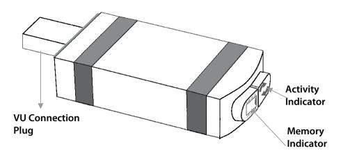
Key to LEDs: Activity – Amber = Active, Green = Complete, Red = Fault.
